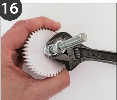
Fasten the large wormgear tight since this will support a lot of weight later
