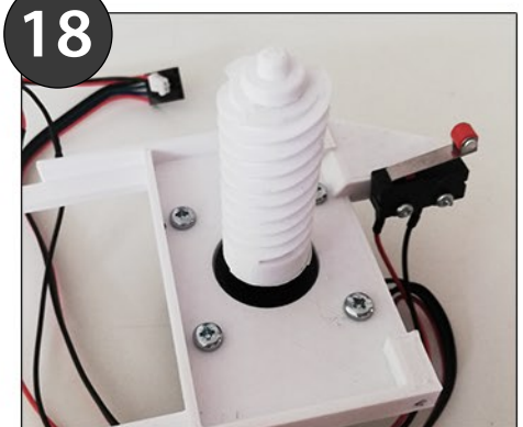
Push the "small wormgear" onto the motor axle
