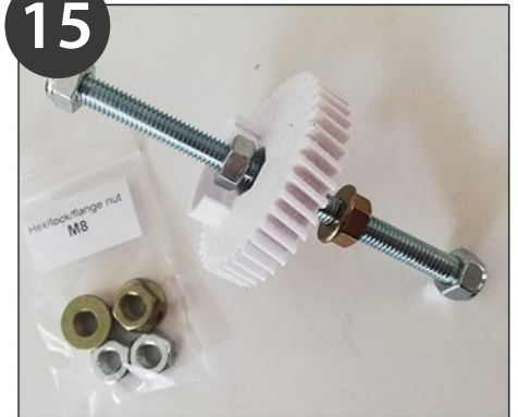
Prepare the threaded rod with 2 lock nuts, 1 hex nut and 1 flange nut like this
