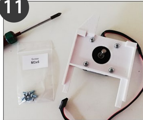
Add the stepper motor to the "motor mount" and fasten with M3x6 screws
