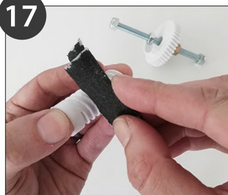
Sand both the gears to remove imperfections
