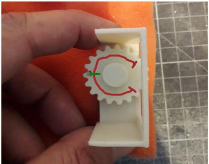
Rotate the elevation sensor to its center position, make a marking with a pen to help keep it correctly adjusted on assembly.
