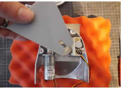
The slits on the main axle for the antenna bracket should be in a 45 degree angle towards the motor as in the photo, which is the center position for the elevation axle.
