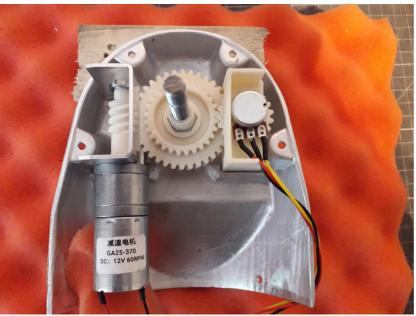
Add motor, axle and sensor like in the photo to the first enclosure side (the one without the rubber cable grommet).
