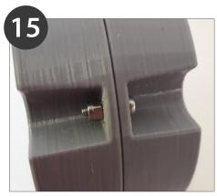
Add the remaining side and fasten together with M3 bolts and nuts.
