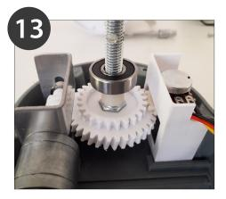
Add motor, axle, sensor, spacer and bearing to the side.
