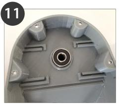
Lay one side on a table and put a bearing in the slot.
