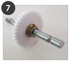
Fasten elevation gear onto the axle with an M8 nut (optionally add loctite/glue)
