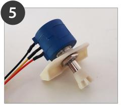
Join the 10-turn azimuth potentiometer with a holder and add a gear to the axle
