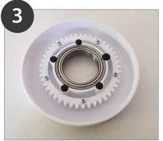
Fasten the large azimuth gear (short 2.2mm screws) and the bearing to the turntable (3x10mm screws)
