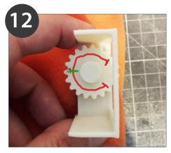
Turn the elevation sensor to its middle position (good to mark it with a pen).
