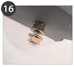
Add two flange nuts on each side of the axle.
