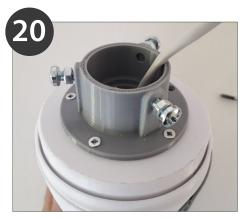
Now fasten the pipe mount to the bottom with 5pcs countersunk screws.
