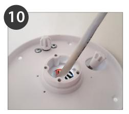
Add the small gear to the azimuth motor axle.
