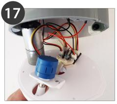
Connect the elevation cables to the patch board.
