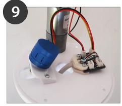
Fasten a motor, control cable and azimuth sensor to the top plate
