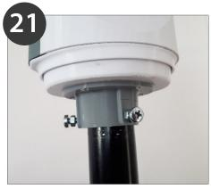
Put the device on top of a tripod with cable running through middle. Fasten.
